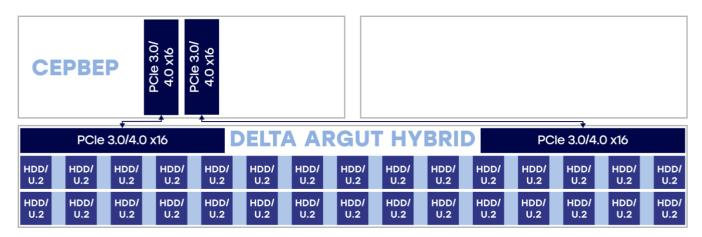
Standard advanced, up to 60 disks 1x Delta Tioga or Delta Serval 1x Delta Sprut 2x Delta Argut Hybrid
